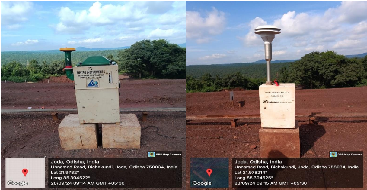
Photo-1 Ambient Air Quality monitoring station at entry and exit gate.
